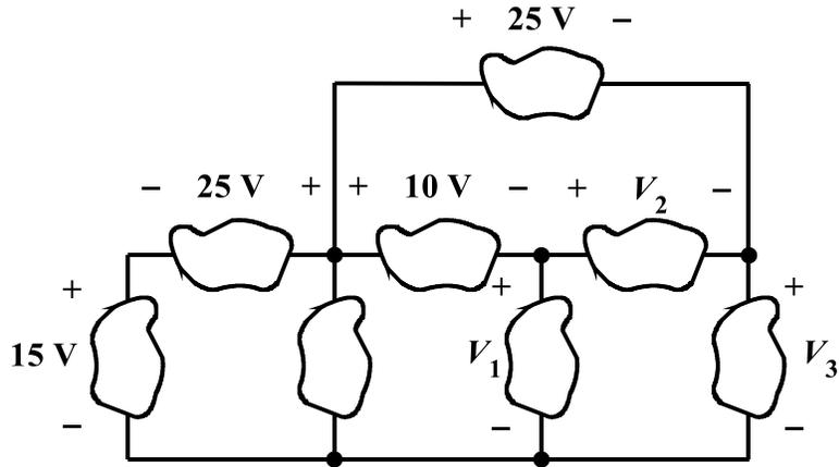
b. Find  $V_1$  and  $V_2$ .
