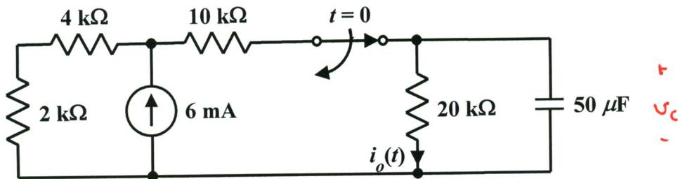
$$V_c(0) = \frac{6}{36} \cdot 6 \text{ mA} \cdot 20 \text{ k}\Omega = 20 \text{ V}$$
