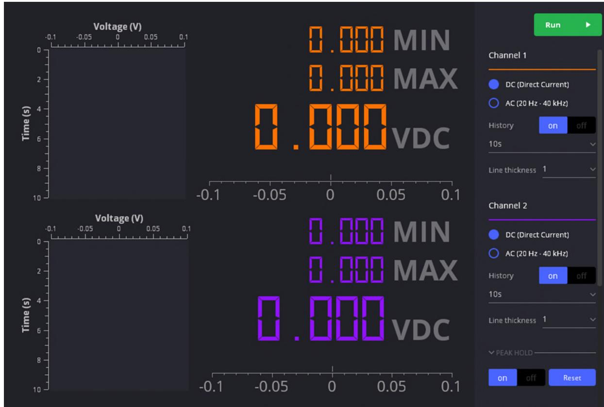
*Figure 6: The Scopy Voltmeter.*
