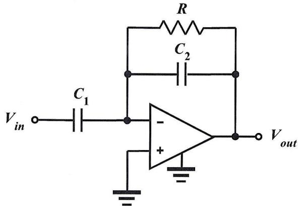
$$\left( \frac{V_{in}}{\frac{1}{j\omega C_1}} \right) + \frac{V_{out}}{R} + \left( \frac{V_{out}}{\frac{1}{j\omega C_2}} \right) = 0 \Rightarrow j\omega C_1 V_{in} = - \left( \frac{1}{R} + j\omega C_2 \right) V_{out}$$
