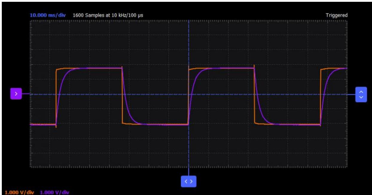
Figure 6. Waveforms for Pulse Width Equal to  $15\tau$ .
