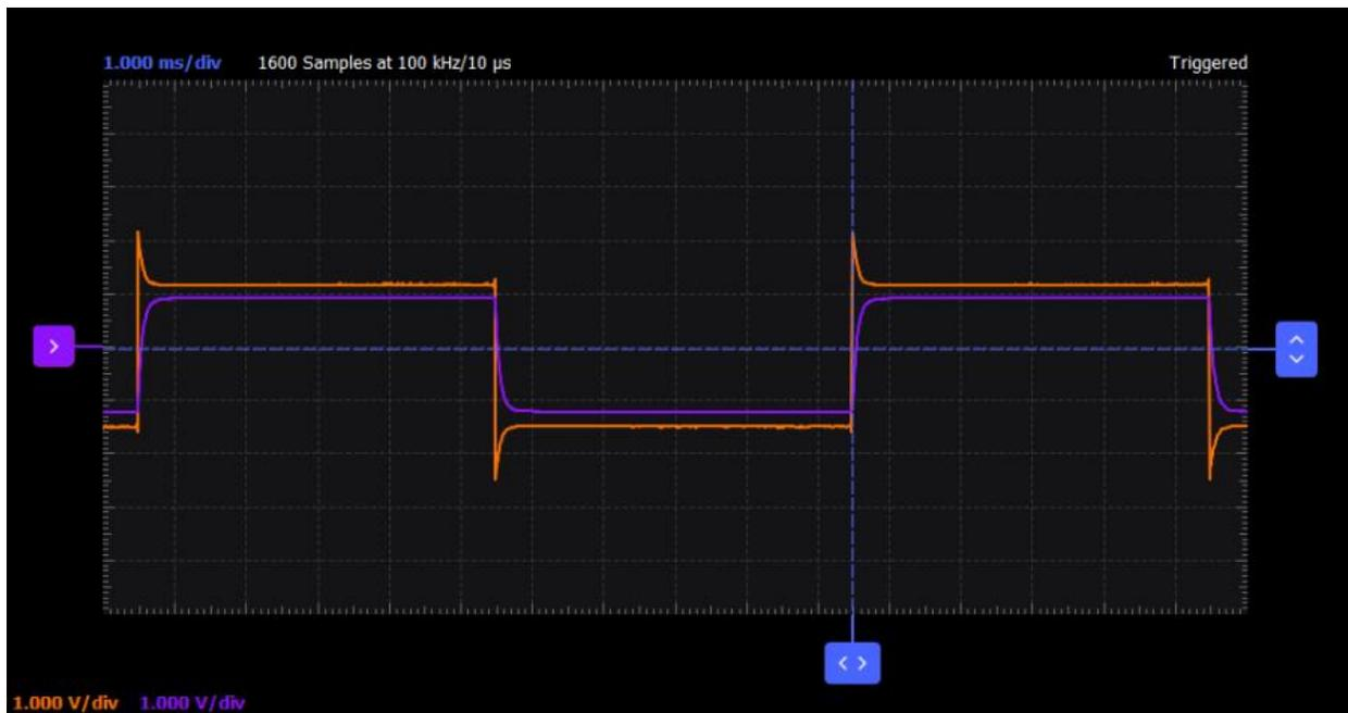
Figure 6. Waveforms for Pulse Width equal to  $5\tau$ .
