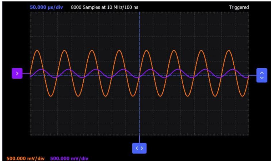
Figure 9: Input and output signals of the  $RLC$  circuit for frequency equal to 10 kHz.
